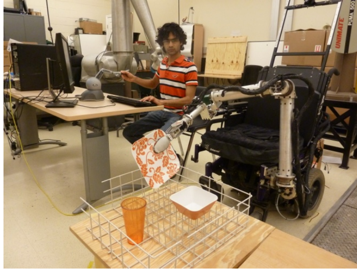
Figure 27: A subject teleoperating to grasp utensils from a dishwasher rack and lay the table (partially visible) on the right
